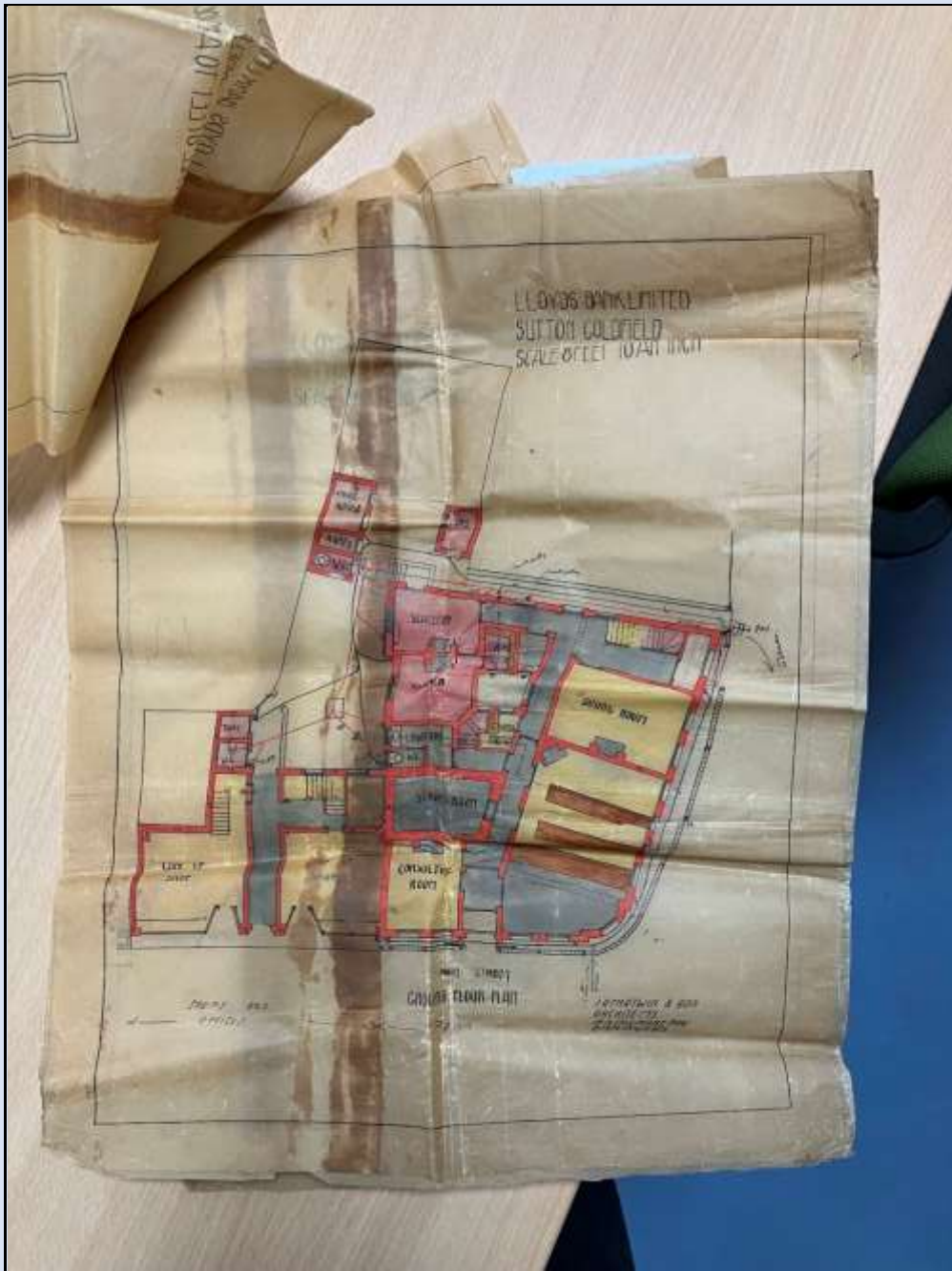
The Ground Floor Plan with a Dining Room and what appears to be a Banking Hall with a Consulting Room, a Strong Room and the usual utilities. Two Lock Up Shops appear to be kept separate from the Banking premises and do not seem to be included in the fascia of the Bank building
