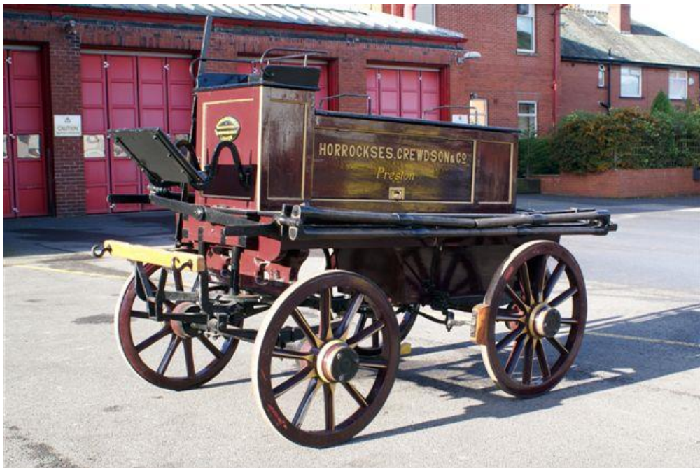
A horse-drawn Shand-Kidd manual fire engine with the water tank mounted on the body of the wagon, which would have also provided seating for the crew. This engine would have been similar in design to the type owned by the Corporation of Sutton Coldfield in 1861 and later. The engine would have required one or two draught horses to haul it and 8 men to operate it using paddles either side of the engine to pump the water onto the fire. Refer to page 12 for details of Sutton Coldfield's fire engine.
