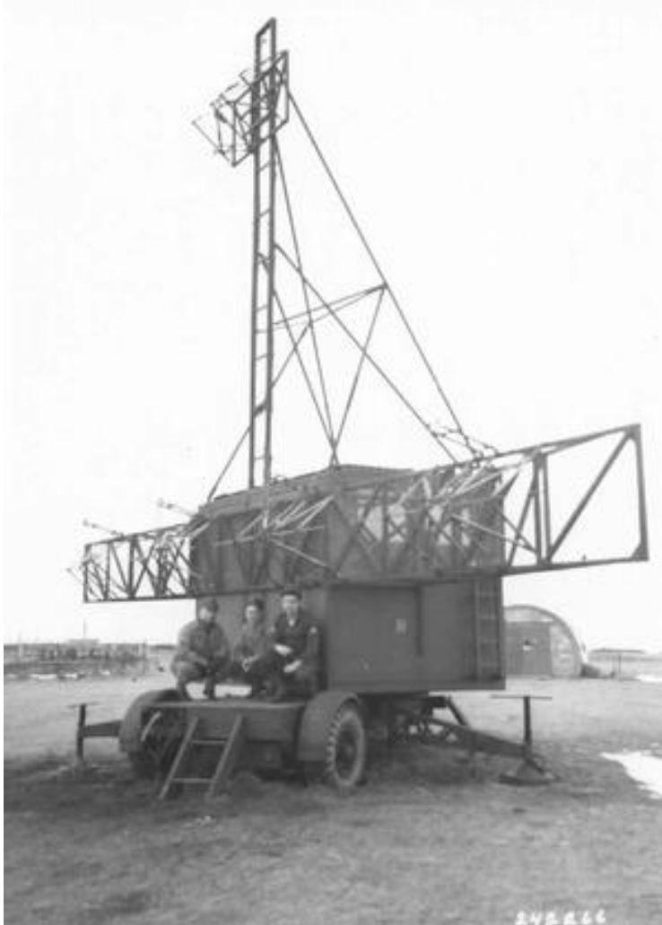
Figure 26. Mobile radar unit of the type used at the Streetly Anti-aircraft Site – a GL Mark 2.
